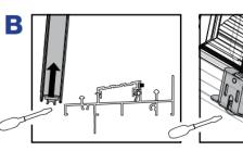
With the panel lifted as high as possible, with a flat head screw driver, lift the bottom spring loaded wheels onto the sill After installing the panel; locate the adjusment screws on the inside face to the panel. Rotate adjustment to lift or lower the panel to ensure ease of sliding.
