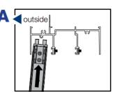
Head Guide will ensure the panel locates in the head correctly and keeps the pressure on the wheels.
