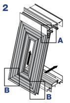
Lift Panel into the channel of the Head Frame
